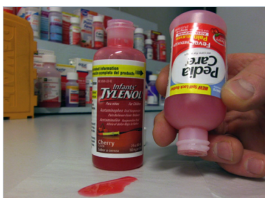
The flow restrictors on products such as PediaCare reduced or eliminated liquid escaping.
